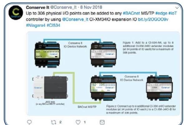
Conserve It Controller adds up to 306 I/O points for BACnet MS/TP.
